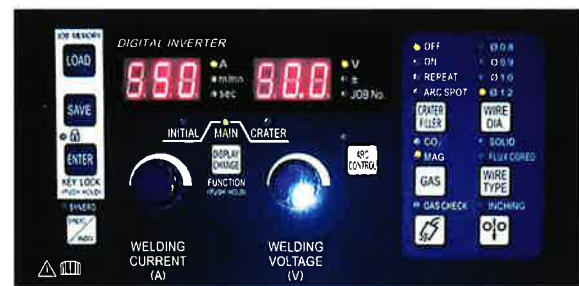
Figure 2 : one knob switch to wire speed display
