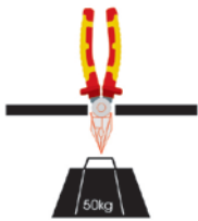
TESTING OF ADHESIVENESS
