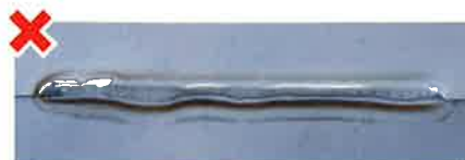
Meandered weld bead due to heat input shortage.
