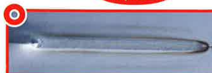
Stable weld bead obtained by fine amp control.
