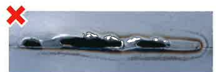
Burn-through caused by excessive heat input
